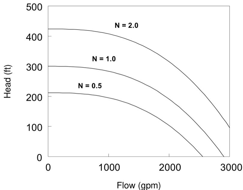
Fig. 5.5 Variable-speed pump curve.
