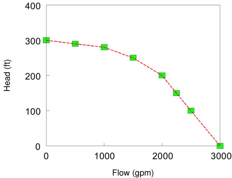
Fig. 5.4 Multi-point pump curve.
