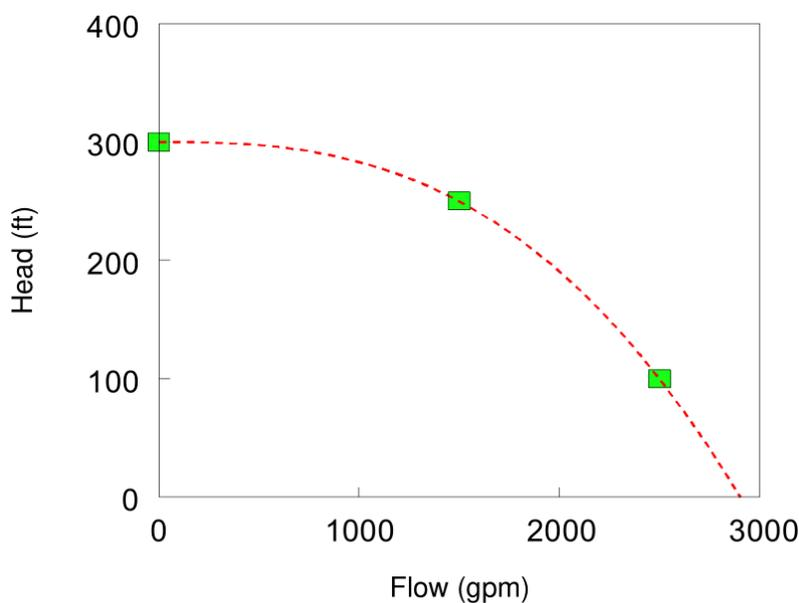
Fig. 5.3 Three-point pump curve.
