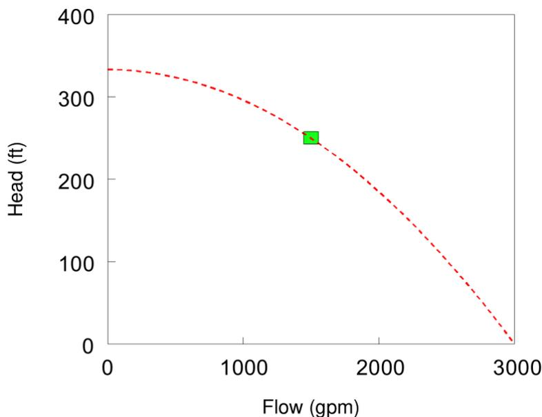
Fig. 5.2 Single-point pump curve.
