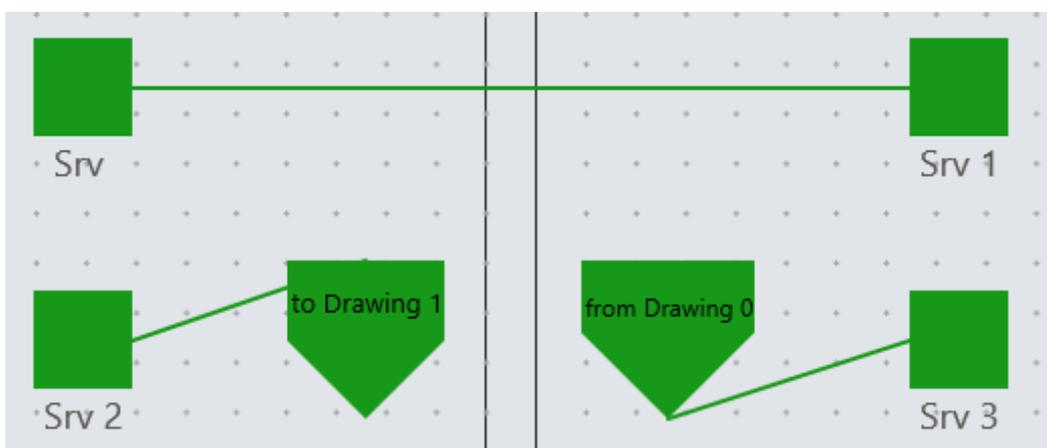
The page reference nodes have no logical function in the simulation and the two link parts both represent the transformed link in the simulation. Simulation display is performed on both link elements. The page location of the page reference nodes can be expressed by **text markup**. The page reference construction is removed from a link by the **Remove page reference** item of the **Transform menu**.
