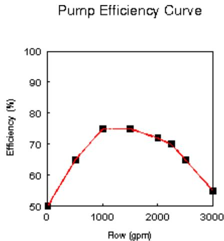
Fig. 5.6 Pump efficiency curve
