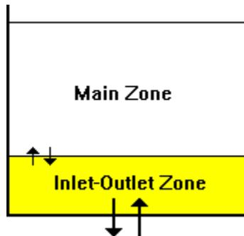
Fig. 5.9 Two-compartment mixing.
