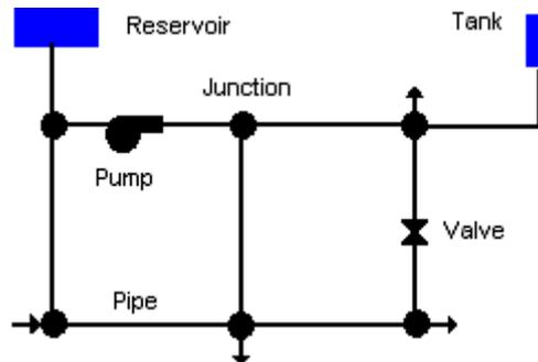
Fig. 5.1 Physical components in a liquid distribution system.
