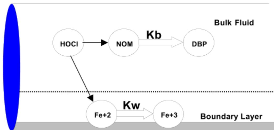
Fig. 5.12 Reaction zones within a pipe.
