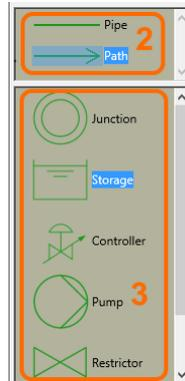
The toolboxes contain one or several default templates. Node and Link objects in the viewport can be stored as new template in the toolbox by the **Create template** command from the **Transform menu** or the contextual menu of a selected object. A new template inherits all properties from the source object. Template properties cannot be changed.
